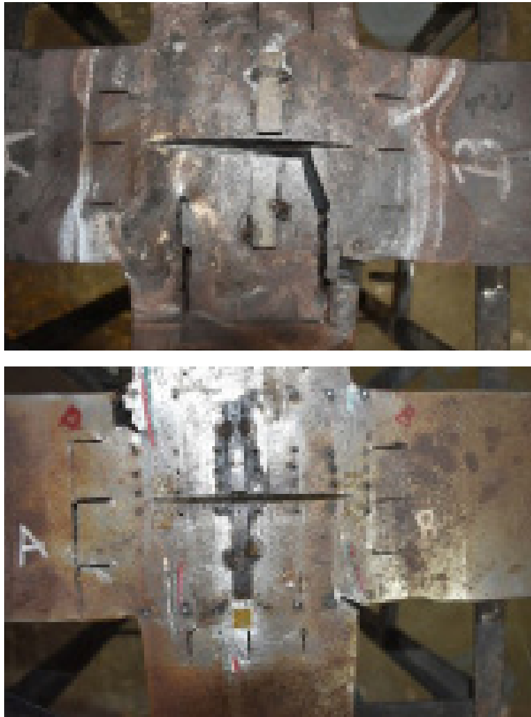
Fig. 9 Cruciform specimens after fracture tests
