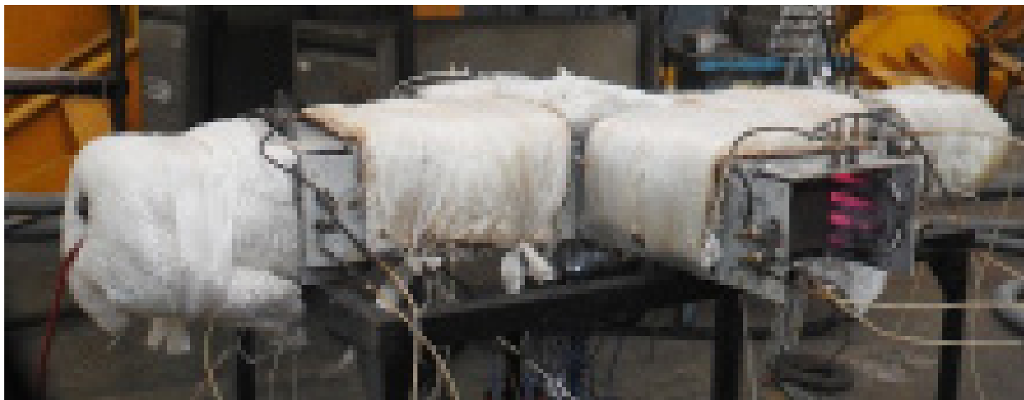
Fig. 5 Cruciform specimen attached with heating coils and wrapped with glass wool measurement
