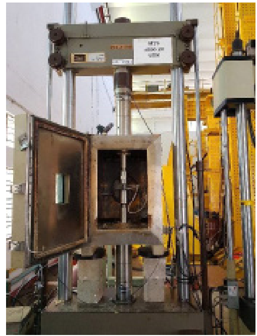
Fig.2: Set- up for tension tests on RPV steel
